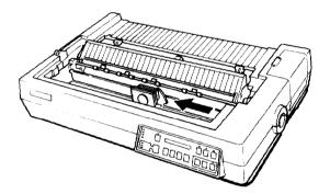
5. Using the enclosed cross-head screwdriver, remove the two red transport screws as shown below.
